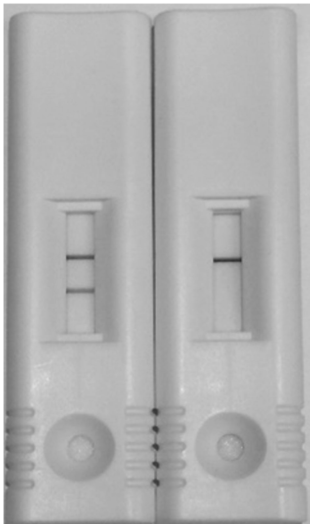
FIGURE 2 A picture of the Amatoxtest 3 showing a negative result (left) and a positive result (right)
